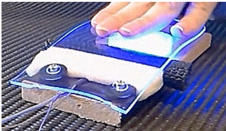
Figure 2. The customised sensor pad; a silicone rubber pad with embedded force sensor and LED.
