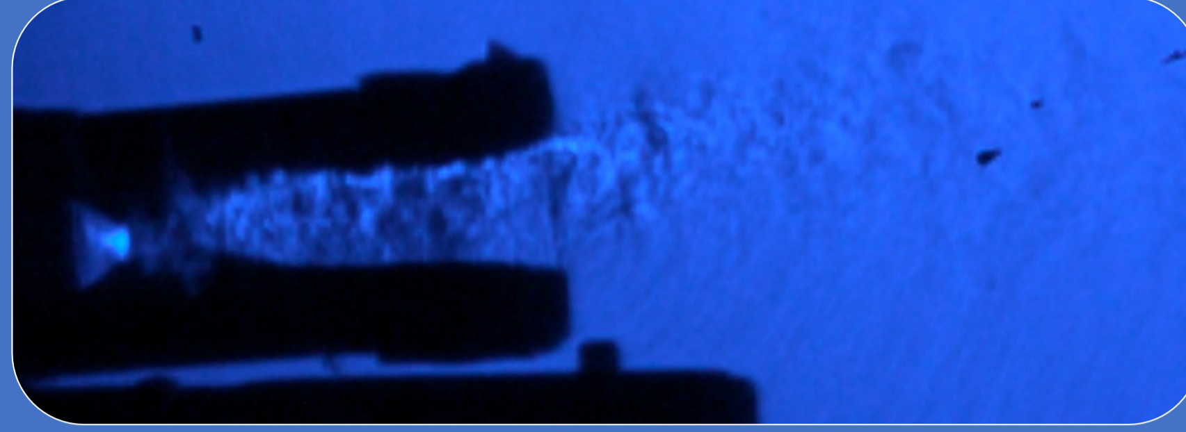
Image 2: Original Nozzle Design, Turbulent flow can be seen inside of the diverging section of the nozzle and flowing out of the exit.
