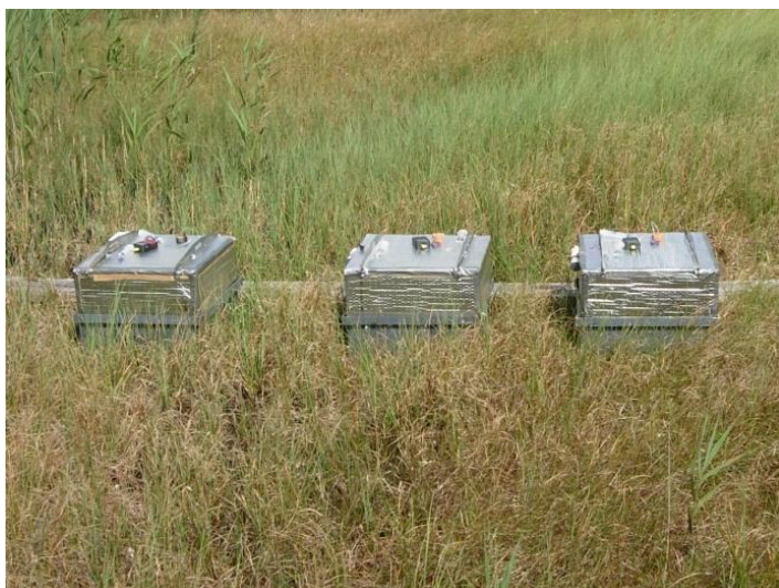
Figure 4.16. Static chambers used for the measurement of carbon dioxide (upper) and methane/nitrous oxide (lower).
