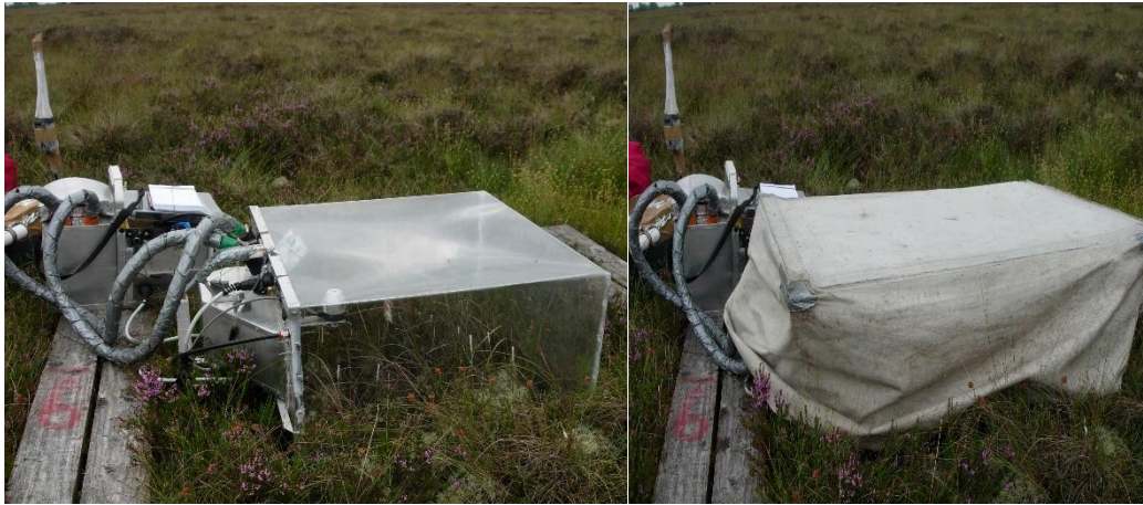
Figure 4.2. Transparent chamber (left photo) and dark chamber (right photo) used to measure carbon dioxide (CO 2 ) fluxes (net ecosystem exchange (NEE) in Moyarwood.
